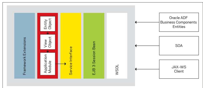
Figure 1: Oracle ADF Business Components service interface architecture
